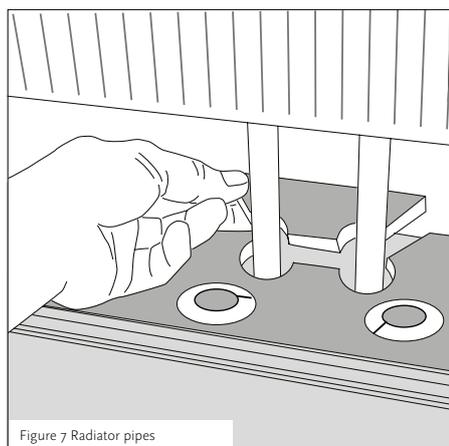
Insert a spacer directly behind the inserted piece to wedge it in place ensuring that the correct sized expansion gap has been left. Leave this in place until the glue has hardened.
